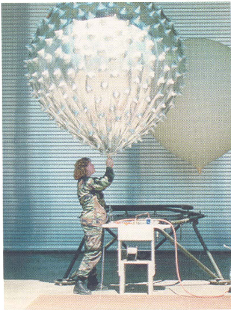
AIC Candie Fuson prepares a jimsphere (weather measurement device) in support of a launch.
