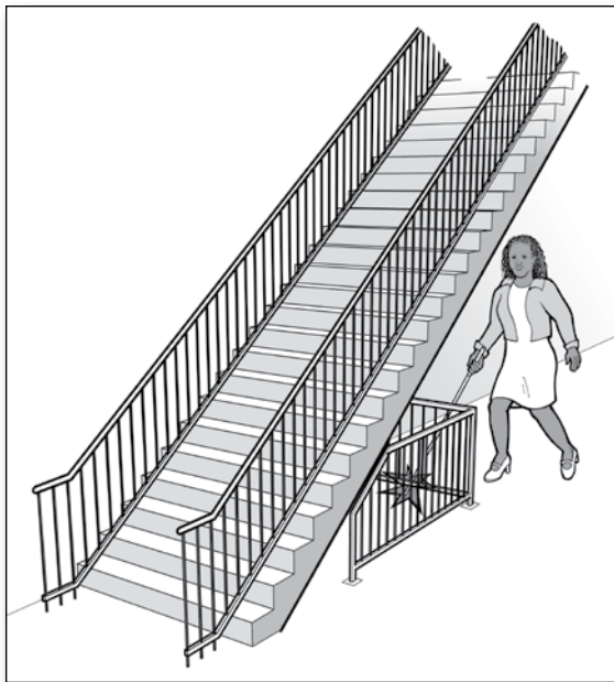
When the underside of a stair is open, it is a hazard to people who are blind or have low vision. Enclosing the area below the stair or installing a cane-detectable barrier helps this woman to stop before hitting her head.
