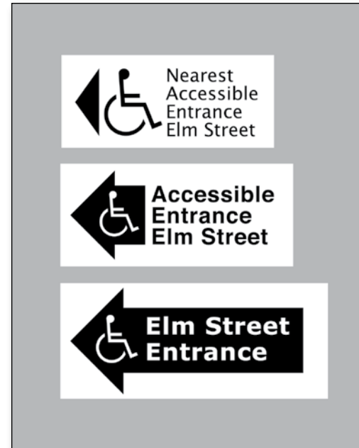
Examples of signs for inaccessible shelter entrances directing people to the accessible entrance.
