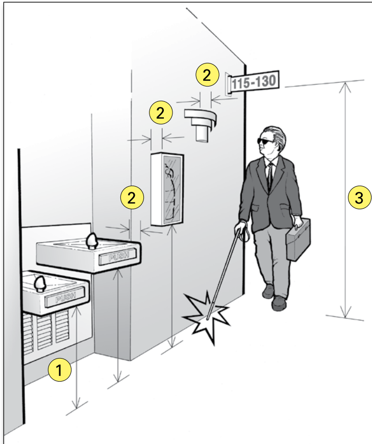
Overhead and wall-mounted objects that may be hazards along a pedestrian route
