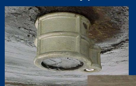
A KINGPIN locking device is an acceptable means of securing a vehicular Type 4 magazine
