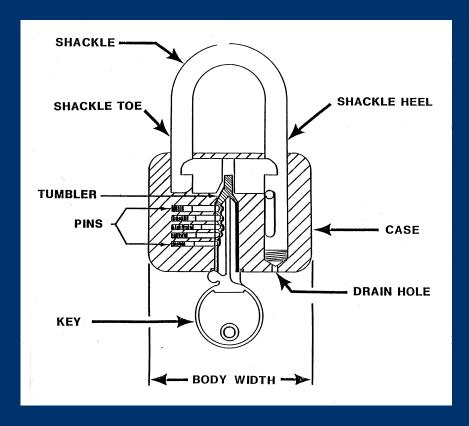
Padlocks must have 5 tumblers and 3/8" case-hardened shackles fastened in separate hasps and staples
