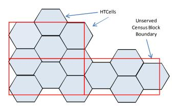
While it is the case that antenna sites would typically lie at the edge of HTCells, for purposes of this model each HTCell would house at least one antenna site. In the case where an existing site structure (e.g., a leasable tower<sup>2</sup>) is used to place a 4G antenna, the actual location of that tower within the HTCell is used in the model. In the case of a 'greenfield' build, the site is assumed to be at the center point of the HTCell.
