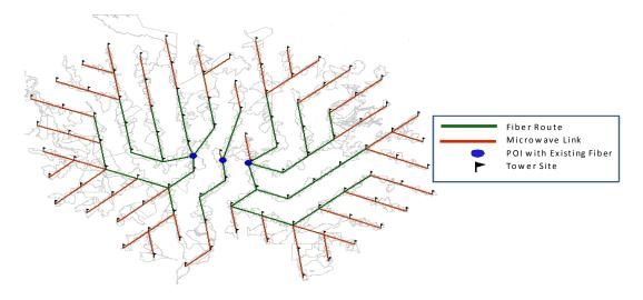
The use of microwave backhaul is subject to a link distance threshold. For this model, the maximum microwave link distance was set at 20 miles. If maximum link distance is exceeded the model assumes the site needs to be served by fiber.
