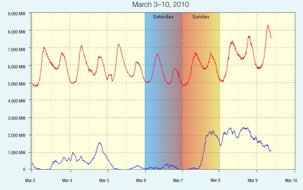
BPA now operates the hydro system to respond to and balance both variations in power loads and unexpected changes — up and down — in wind power output.
