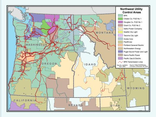
BPA is the balancing authority responsible for maintaining a constant balance between the power load and power generation in the area shown in teal. (A balancing authority is also known as a control area.) Most of the wind power on line and planned for the Pacific Northwest is clustered in BPA's balancing authority at the eastern end of the Columbia River Gorge. However, 80 percent of the wind power in BPA's balancing authority area serves loads in other utilities' balancing authorities.
