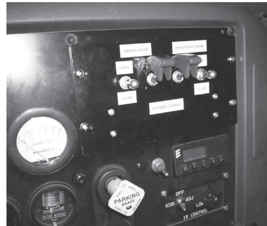
This EDAS's switches have been installed and mounted to the vehicle's dashboard. It fits into an existing pocket, which saves space. By placing it in a central location, both driver and passenger can operate the system. (U.S. Army TARDEC photo by Mark Fuller.)
