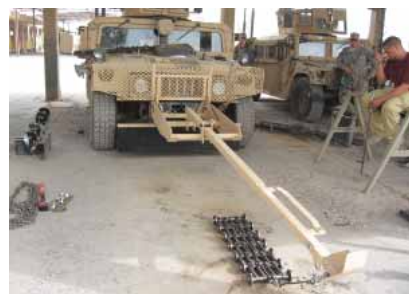
A team installs the Wolf Claw on an up-armored HMMWV in theater. The Wolf Claw attaches directly to the HMMWV and to any SPARK VCMB. Adjustable to various standoff lengths, it is a useful tool that is defeating IEDs. (U.S. Army TARDEC photo by Andy Scott.)
