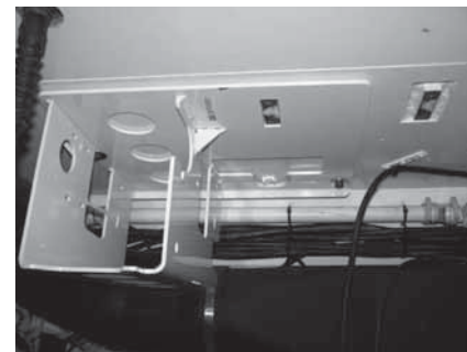
The OSRVT A-Kit ceiling brackets allow Soldiers to mount the urgently needed technology in an out-of-the-way place. By doing so, they still have access to the technology's full scope but are able to safely egress the vehicle in an emergency. (U.S. Army TARDEC photo.)
