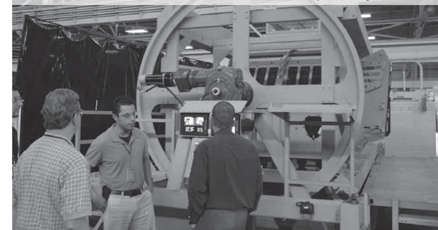
The MET, which provides Soldiers invaluable training on how to react following a vehicle rollover, was showcased at the TARDEC Prototype Integration Facility (PIF) Open House June 23, 2009. Warfighters now feel safer and more prepared for the common, dramatic event. Shown here is the front of the MRAP mechanism. (U.S. Army TARDEC photo.)
