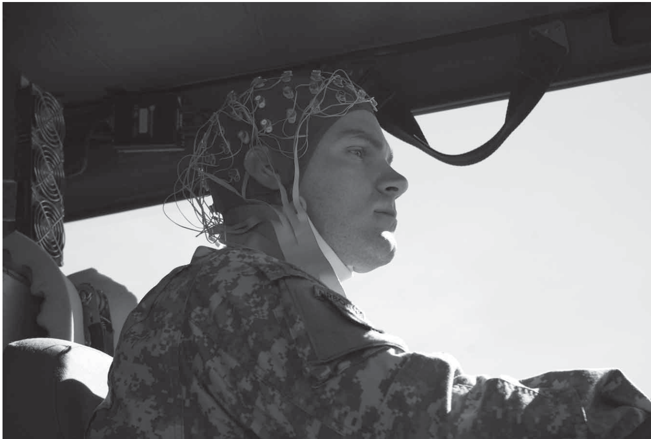
During the testing, Soldiers wore an ARL HRED neuroergonomic cap to record brain waves related to their reactions to driving autonomously. Neuroergonomics, the study of brain and behavior at work, combines neuroscience and human factors. Through the ARL HRED and TARDEC engineering partnership, test results indicate that CAST will decrease driver workload.
