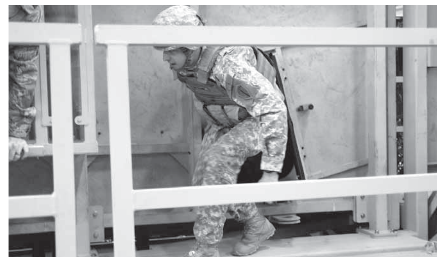
A Soldier exits the MET, simulating a vehicle on its side, during trainer evaluation testing at TARDEC. The MET is capable of conducting egress training at 90- and 180-degree positions.
