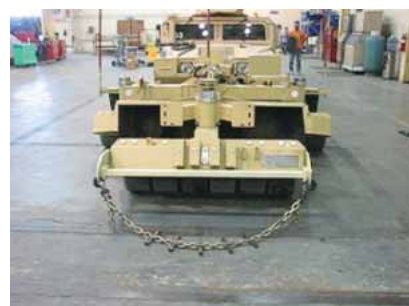
A Wolf Collar is attached to the front of an up-armored HMMWV's SPARK roller. (U.S. Army TARDEC photo by Andy Scott.)
