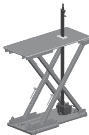
A CAD drawing of an MRAP Cougar variant GRS. TARDEC design engineers began the entire restraint process by physically measuring bolt hole locations in each MRAP vehicle variant. (U.S. Army TARDEC drawing.)
