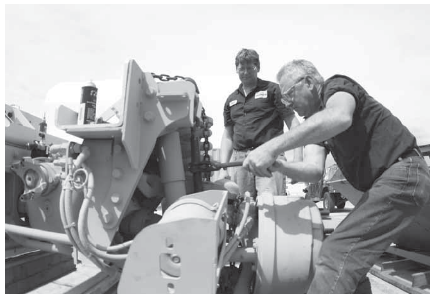
An Oshkosh Truck Corp. test technician prepares a new independent suspension system to be installed on an MRAP as an Oshkosh senior test technician observes the process June 3, 2009, at the Combat Center's Exercise Support Division maintenance bay. Detecting mechanical faults in suspension systems by comparing measured operational vibrations could revolutionize vehicle component diagnostics. (U.S. Marine Corps photo by CPL Margaret Hughes.)
