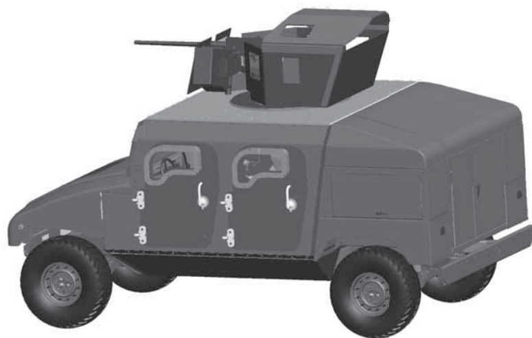
Lightweight vehicles, like this artist's rendering, are more fuel efficient and have fewer logistics problems than MRAP vehicles. As a result of the LVUPS's design and prototyping processes, such vehicles will be able to withstand greater threats than current vehicle systems. (U.S. Army TARDEC drawing.)
