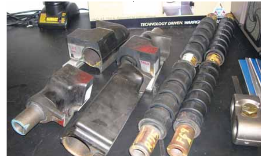
EIP testing has discovered that bushings undergo 55-percent deterioration after assembly, which can lead to track and component failure. TARDEC researchers are trying to create bushings made of more durable, consistent material that will improve track durability and performance in harsh terrain. (U.S. Army TARDEC photo by Chris Williams.)
