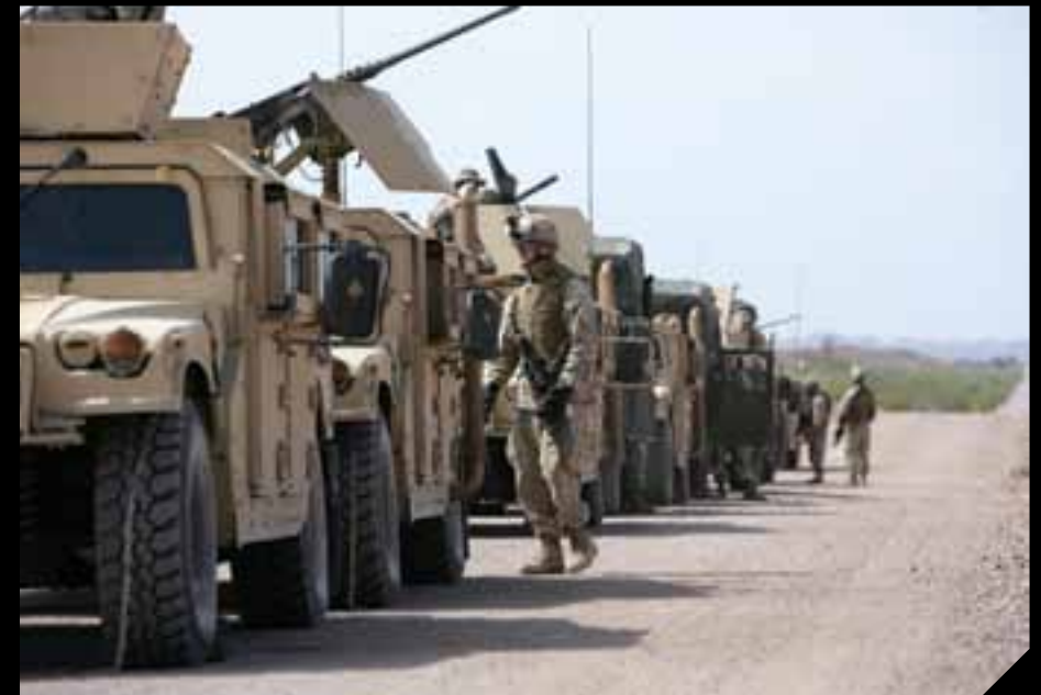
FED Program engineers used the M1114 HMMWV Frag 5 as the baseline vehicle for benchmarking threshold requirements for the FED vehicle. Systems engineers are integrating available technology to maximize fuel economy. (U.S. Army photo by SGT Benjamin R. Reynolds.)
