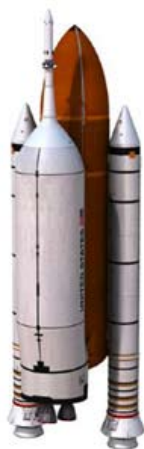
Figure 5.2.2-2. Shuttle-Derived Sidemount Launcher. Source: NASA
