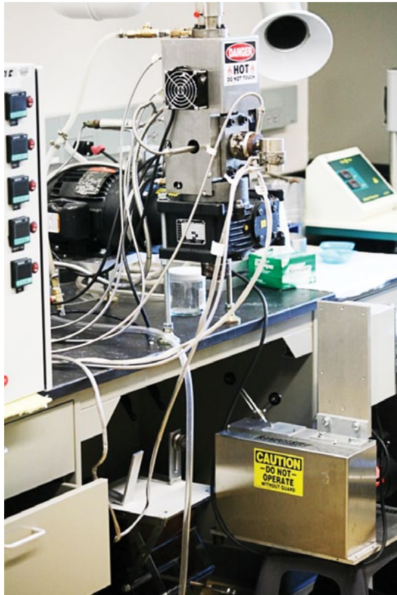
Instrument that extrudes biodegradable polymer into bone pins (RCCC).
