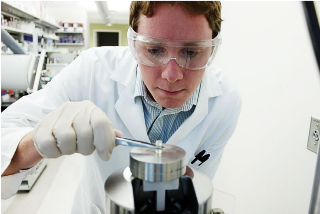
WFPC researcher Allan Henslee, a Rice University graduate student, prepares to characterize the compressive mechanical properties of a material designed for bone regeneration.
