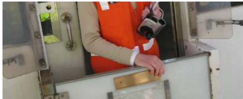
Figure F-5. Bumped Out Dutch Doors Can Reduce Twisting and Turning for Collectors
