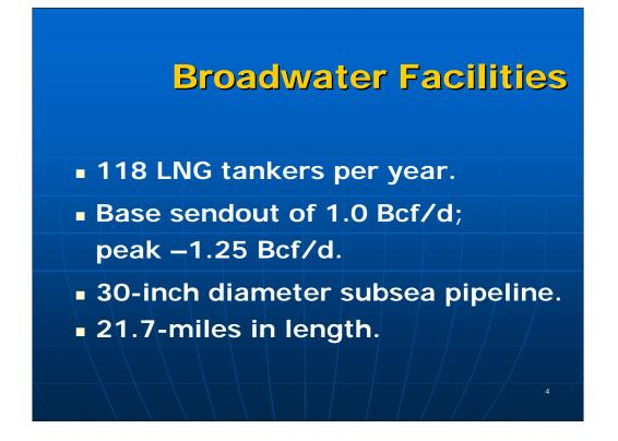
The FSRU is approximately 1,215 feet long, 200 feet wide, and extends approximately 80 feet above the waterline. The FSRU will have a receiving berth for unloading LNG carriers, storage tanks, vaporization facilities designed with a base capacity of 1.0 Bcf and a peak capacity of 1.25 Bcf, gas treatment facilities, power generation, and a crew accommodation area.
