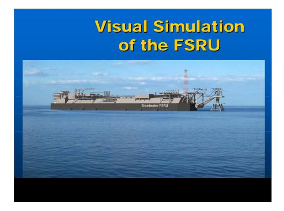
Broadwater Energy's proposed LNG terminal will consist of a floating storage and regasification unit or FSRU that includes a yoke mooring system attached to the bow of the FSRU that will "moor" the FSRU to a fixed tower. The FSRU will be located in Long Island Sound approximately 9 miles off the shore of Long Island, New York and 10.2 miles from Connecticut in waters approximately 90 feet deep.
