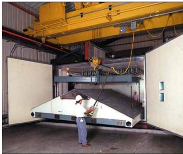
A test attic being loaded into the BTRIC Large-scale Climate Simulator
