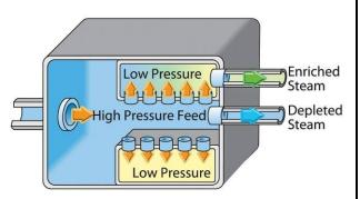
with higher molecular weight. Because the walls of the vessel are semi-permeable, more of the lighter molecules flow through the wall than the heavier molecules. As such, gas that passes through the walls of the vessel is slightly enriched in the lighter isotope.
