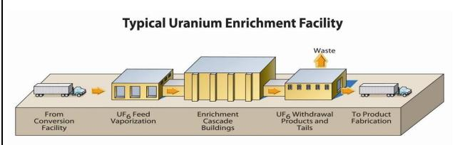
The uranium fuel cycle begins by mining and milling uranium ore to produce  $U_3O_8$ , also known as "yellow cake," which is then converted into uranium hexafluoride (UF<sub>6</sub>). The UF<sub>6</sub> is then enriched before being made into nuclear fuel. Throughout the global nuclear industry, uranium is enriched by one of two methods: gaseous diffusion or gas centrifuge. A third method – laser enrichment – has been proposed for use in the United States.
