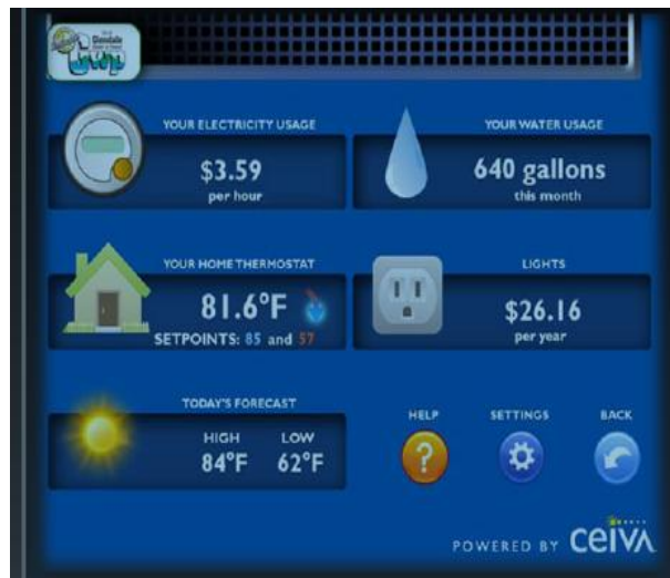
A digital photo frame is part of Glendale Water and Power’s (GWP’s) in-home display pilot that is enabling customers to track their usage without having to go online to access the data.
