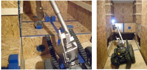
Directed Perception and Grasping Dexterity Test Method
