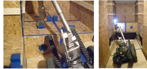
Directed Perception and Grasping Dexterity Test Method
