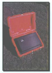
Q730 system with the cover open. The sealed polyethylene enclosure, standard on all Quanterra products, is water tight.
