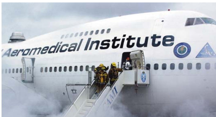
The 747 Aircraft Environment Research Facility being utilized for evaluation of simulated emergency aircraft evacuation.
