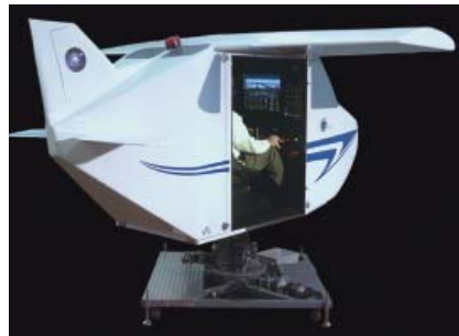
CAMI's General Aviation Pilot Trainers teach pilots to recognize and manage the symptoms of spatial disorientation.
