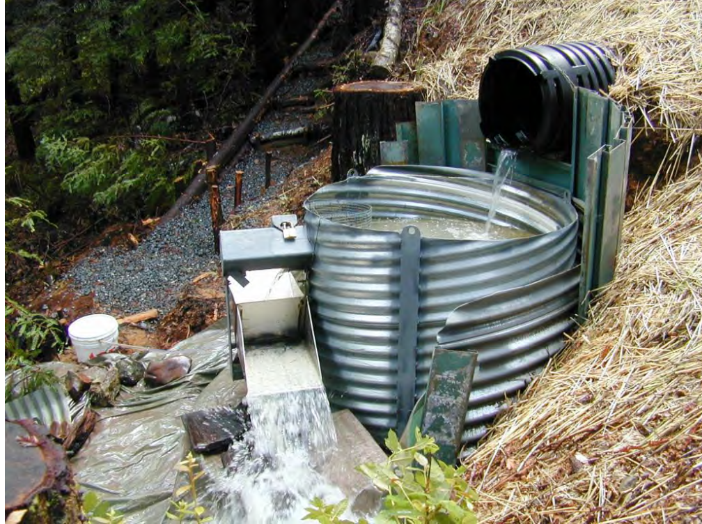
Figure 2 —Site 10 in operation with coarse sediment collection tank, tipping bucket, and suspended sediment sample bucket with tubing.
