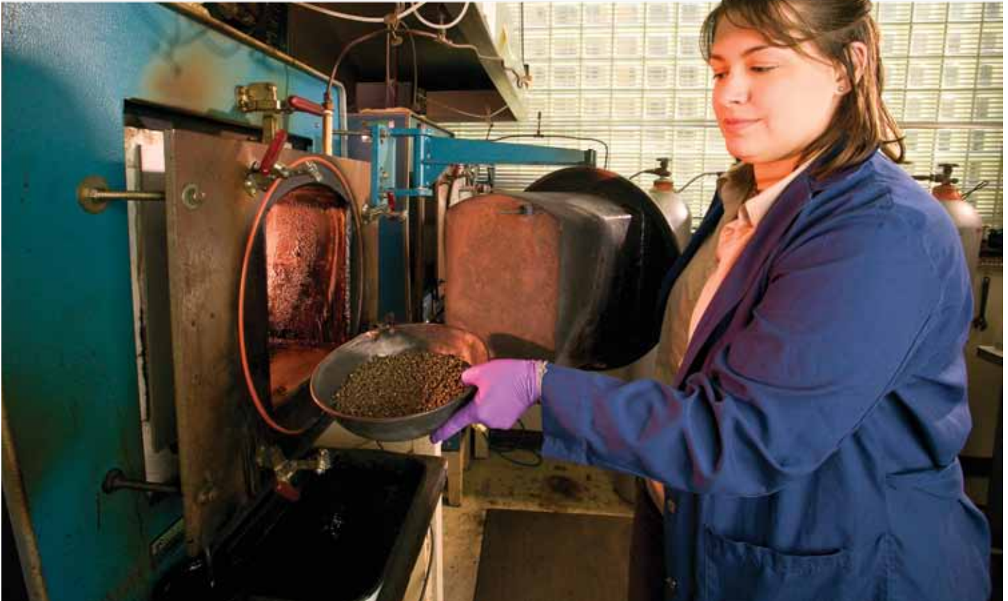
In New Orleans, technician Renee Bigner places poultry litter pellets into a furnace to make biochar via slow pyrolysis.
