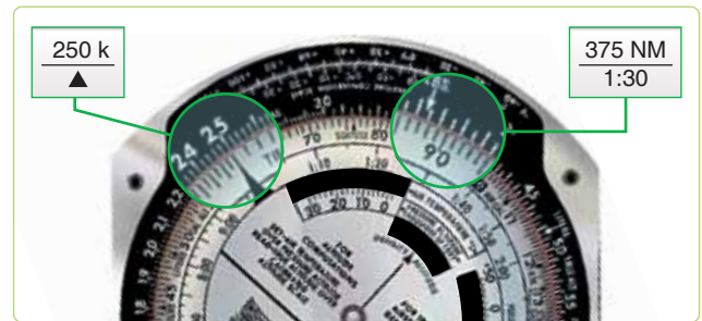
Figure 4-17. Solving for speed when time and distance are known.
