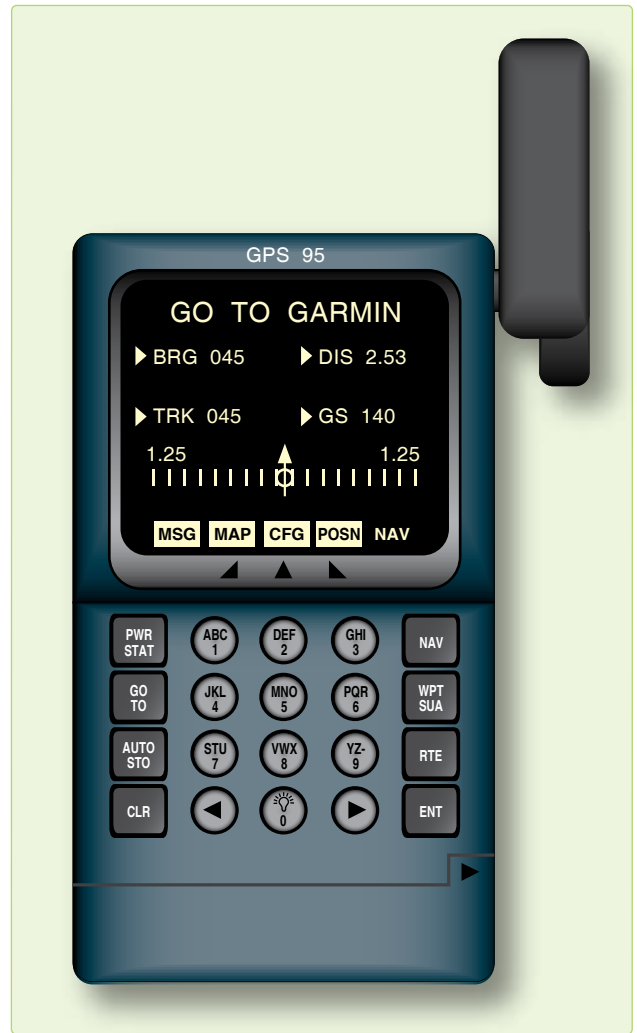
Figure 16-11. Handheld user equipment set.
