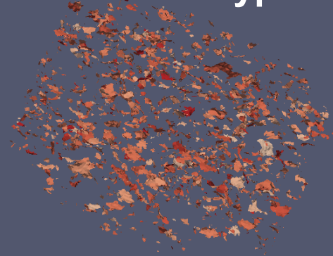
Extraction of one Grain Boundary Interface Type
