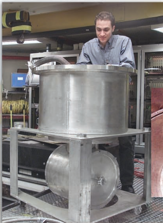
Konstantin Lokshin works on the apparatus we used to study hydrogen clathrate. The inset is a closeup of the high-pressure cell in which the clathrate formed.
