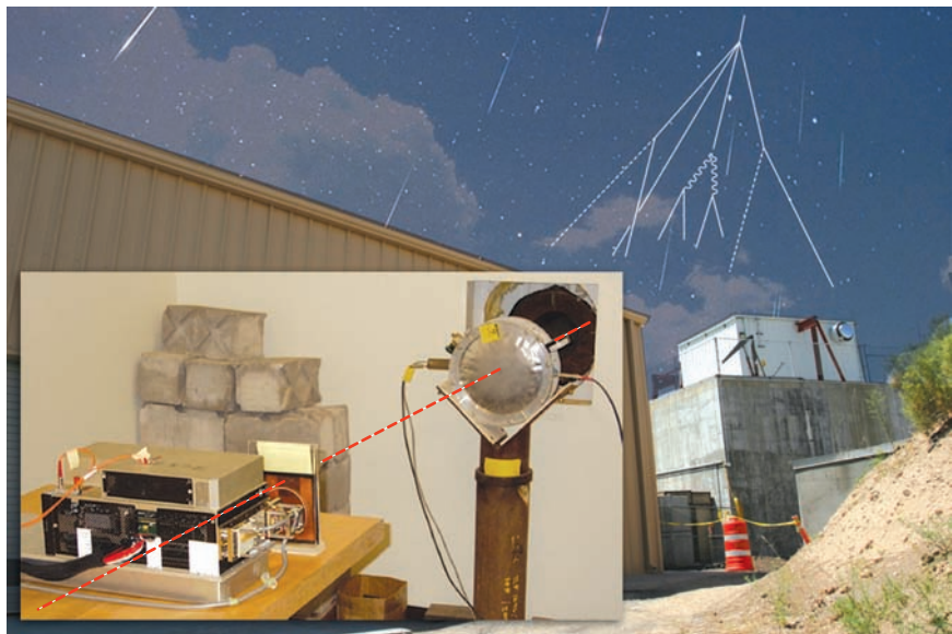
Figure 7. Testing Semiconductor Electronics at the ICE House At the ICE House, Honeywell and NASA placed a flight control system in the neutron beam (inset) to determine how well the system would recover from upsets induced by atmospheric neutrons.
