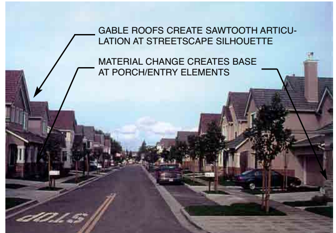
Desirable: Gable Roofs add variety to roof silhouette along street scape creating "sawtooth" appearance.
