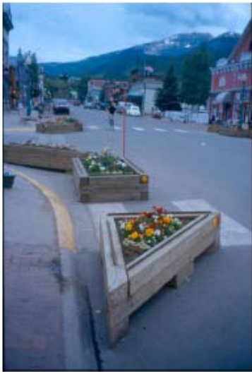
Exhibit 4.22: Temporary summer curb bulb-outs in Crested Butte, Colorado, improve pedestrian crossings on wide streets. 19
