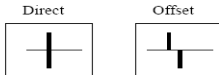
Figure 25. Illustration of a direct versus an offset intersection.
