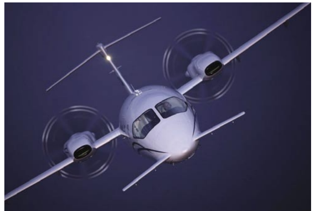
Figure 5-14. The Piaggio P180 includes a variable-sweep canard design, which provides longitudinal stability about the lateral axis.
