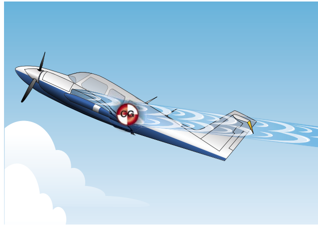
Figure 5-11. Airplane with a T-tail design at a high AOA and an aft CG.
