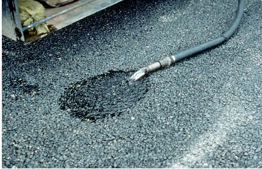
Figure 4-3. Drainability and texture of finished ATPB.
