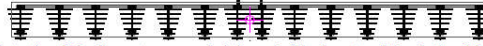
Illustration of a localizer antenna array depicting each of the elements and the selection of the HSP and Vertical Point #1.
