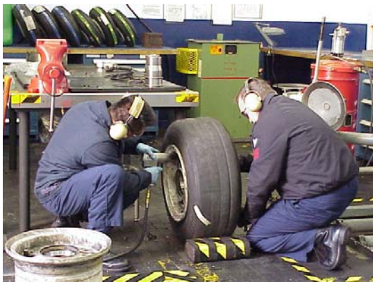
Figure 3: Removing lug nuts (photo from AIMD SD)
