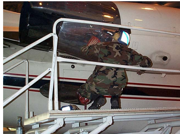
Figure 6: Polishing from a platform
