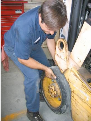
Figure 6: Changing a forklift tire
