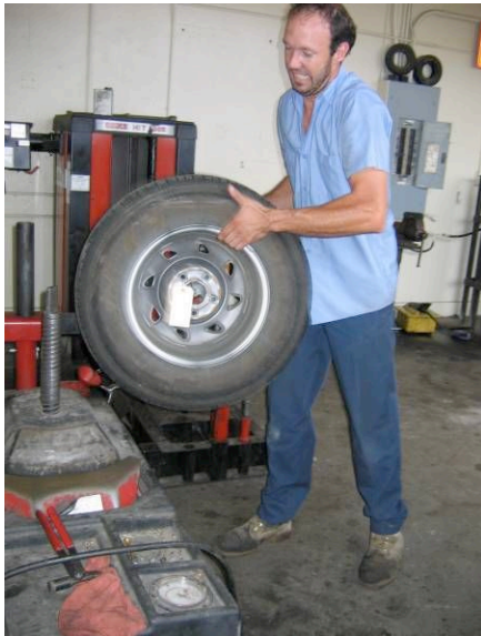
Figures 7: Lifting tire onto machine
