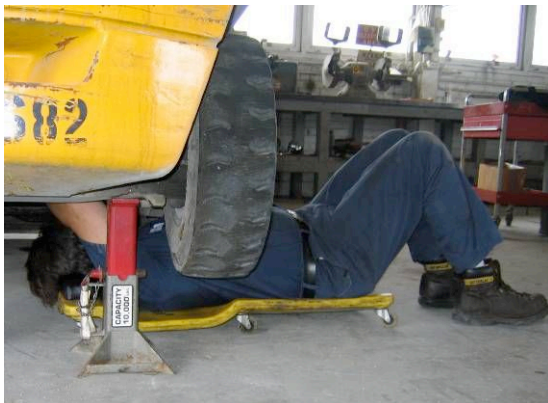
Figure 1: Working under a vehicle
