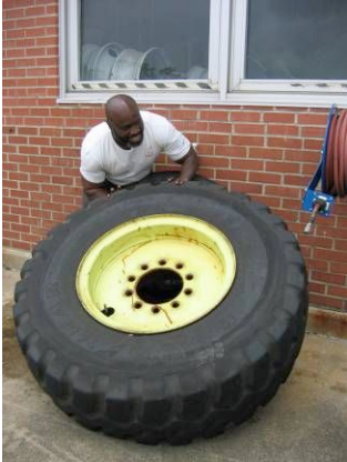
Figure 9: Lifting a P19 tire
