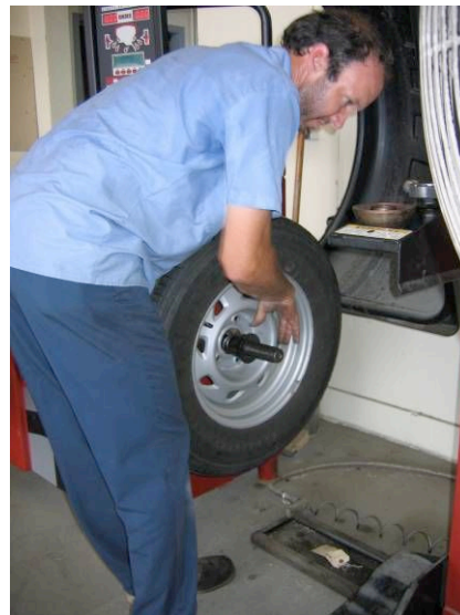
Figure 8: Holding tire at balancer
