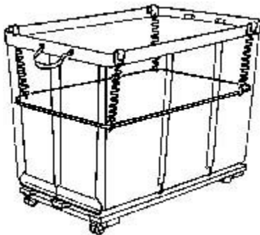
Mail Hamper with Spring Platform (Platform moves independently)
