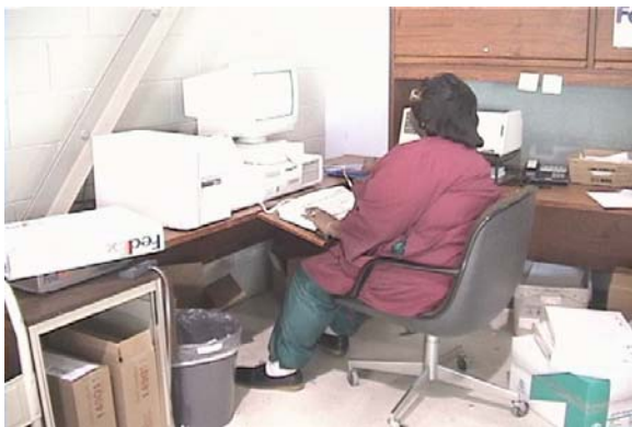
Figure 8: Seated computer workstation (note positive tilting keyboard, tall monitor height, and chair with 4-star base)
