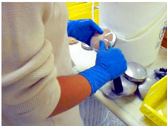
Figure 7: Operator using a knife to remove pads
