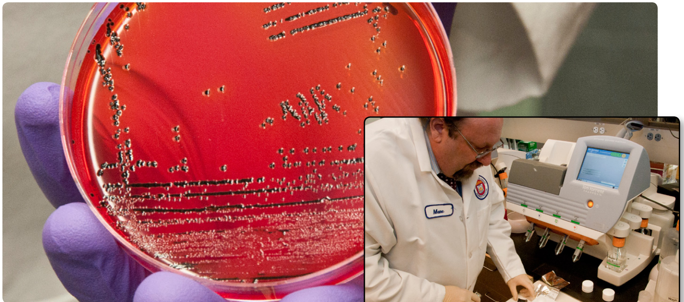
Salmonella bacteria, shown here in a petri dish, are a major cause of foodborne illnesses. Scientist Marc Allard uses a genome sequencing machine being tested for field applications to rapidly identify the genetic makeup of disease-causing bacteria. For more photos of scientists at work in FDA’s Center for Food Safety and Applied Nutrition, visit www.flickr.com/photos/FDAphotos .
