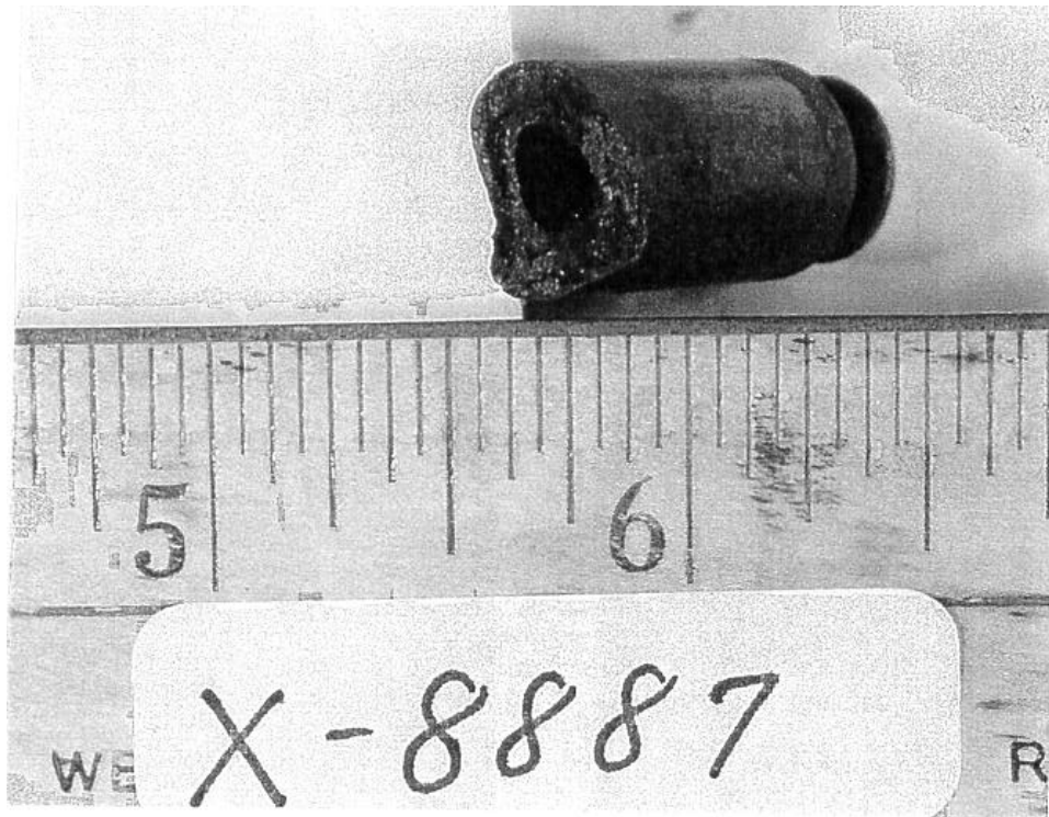
Figure E-16: Perspective view of the fractured dowel pin showing the fracture face extending through the drilled hole within the center of the pin.
