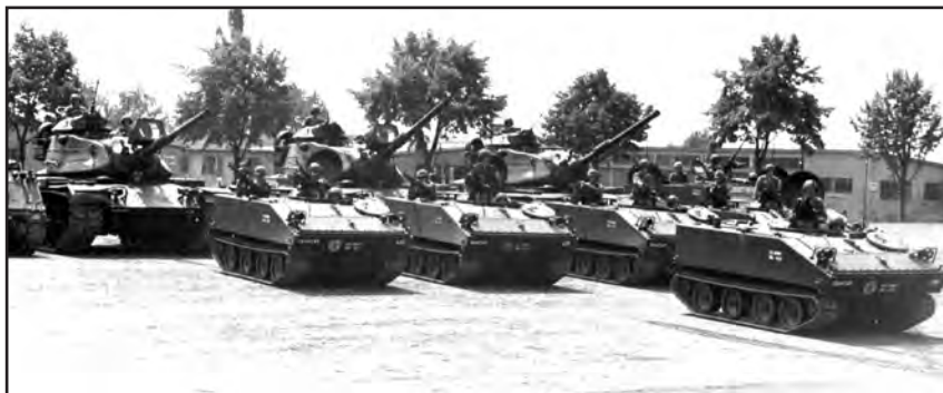
Figure 77. Cavalry platoon in Germany illustrating the mixed composition of M60 tanks and M114s.
