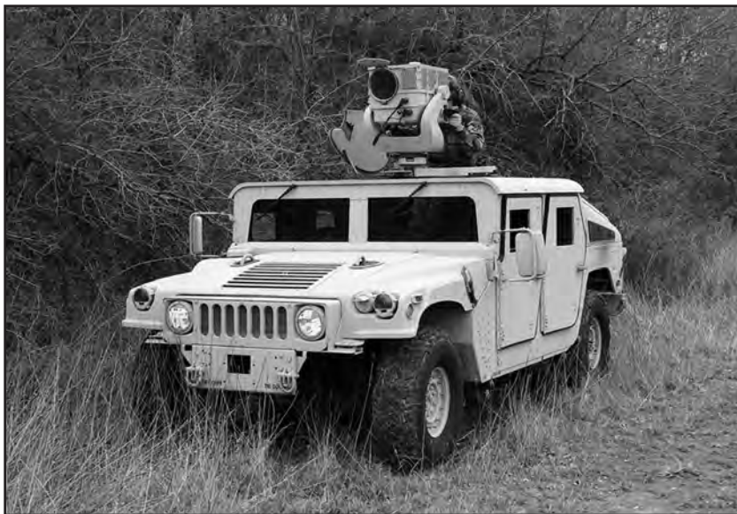
Figure 98. The LRAS3 mounted on a HMMWV.
