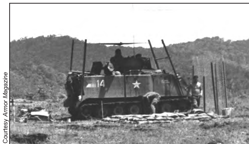
Figure 71. M113 behind chain link RPG screen intended to detonate prematurely incoming projectiles.
