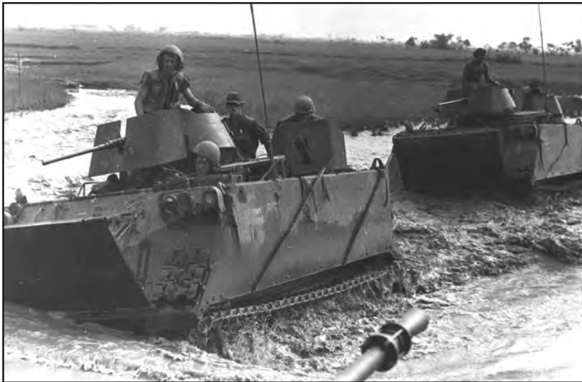
Figure 64. The M113's mobility made it invaluable during the rainy season in Vietnam and in crossing the many small waterways. Here ACAVs traverse a flooded area.
