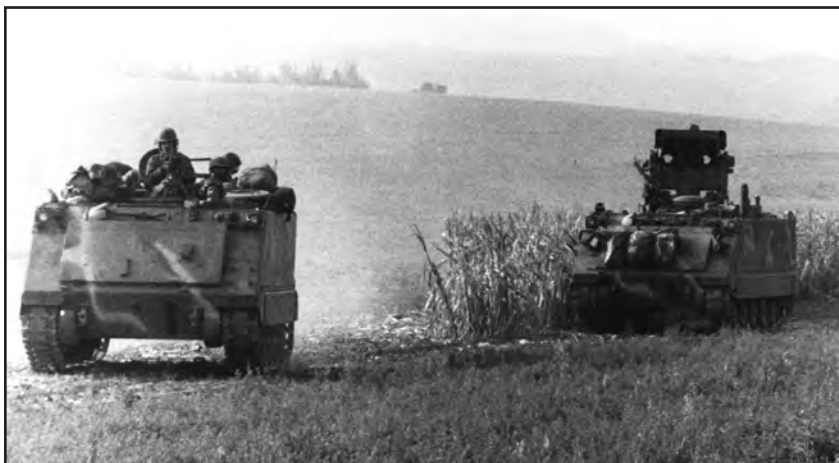
Figure 85. Scout section on the move—an M113 and an ITV working together.
