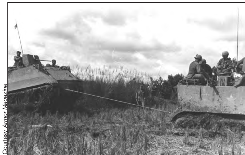
Figure 59. Use of an M113 to recover another—a common activity in South Vietnam and necessitated by the terrain conditions.
