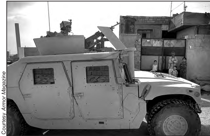
Figure 126. M1114 Up-Armored HMMWV with improved protection for the gunner.
