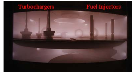
Figure 3.2: Plasma deposition of low-friction coatings on truck components
