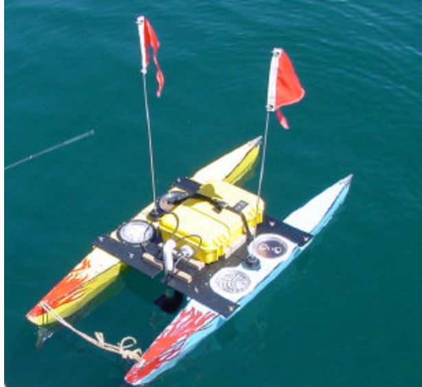
Figure 1. Autoboat with echosounder (from Hawks-Johnson 2003). This approach will be applied in the inshore waters of Washington and Alaska.
