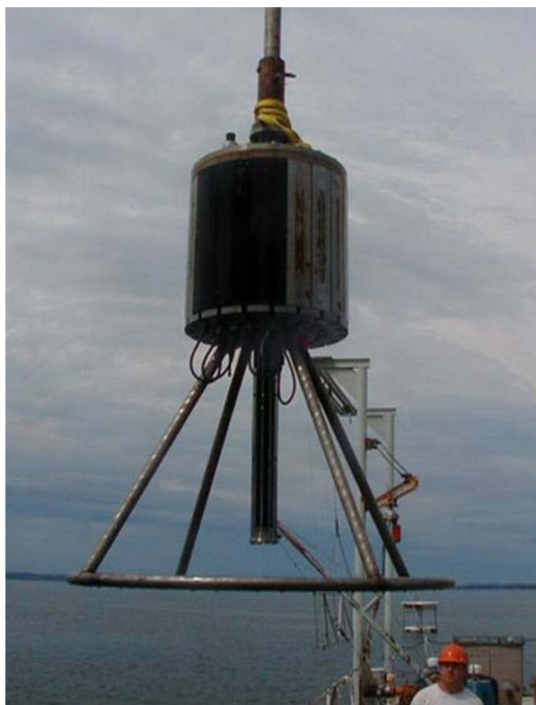
Figure 9 - Pictures of the IMAPS sonar head. The picture on the left shows it during preliminary testing when only 10 receive sensors were installed. The picture on the right is nearly fully assembled missing only the transmit line array.
