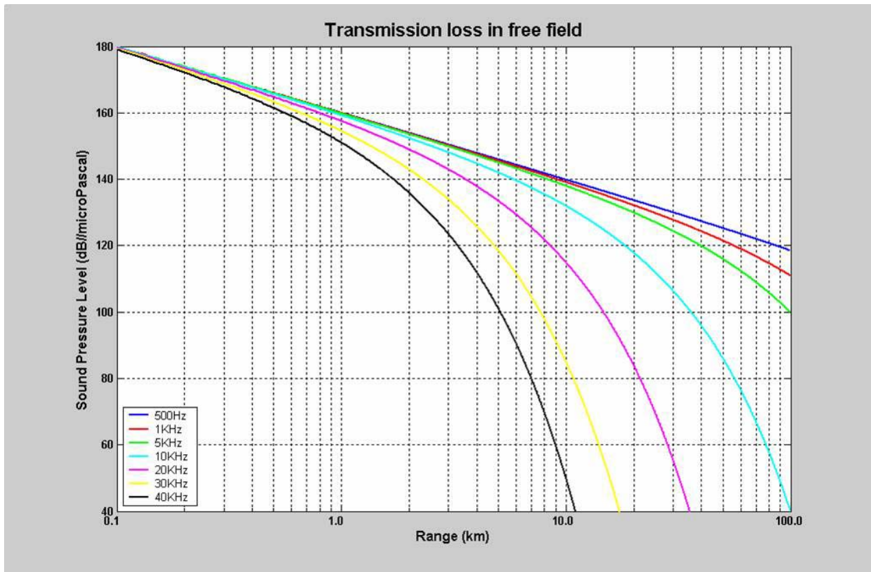
Figure 13 - Sound pressure level versus range for various frequencies and a source level of 220 dB re 1 \mu Pa at 1 m. This assumes spherical (free-field) spreading plus absorption. In most realistic cases, scattering from the boundaries will increase absorption at the higher frequencies. At 20 kHz, the lowest frequency of operation of the whale finding sonar, the sound dies away rapidly beyond several km.
