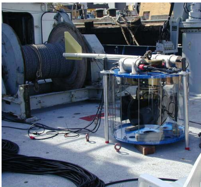
Figure 7 - The MAST (Marine Mammal Active Sonar Test) mechanical system. It is a version of HF/M3 that is not integrated in SURTASS LFA and is meant to be deployed from a stationary vessel.
