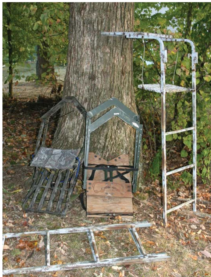
The two tree stands on the left are climbing-type while the one on the right is referred to as a ladder stand. While the ladder stand design is statistically safer, all require the use of a safety harness to prevent a fall.
