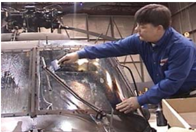
The windshield tear-off is being applied to a Blackhawk helicopter by Steve Fricker of United Protective Technologies at Fort Eustis, Va. Photo by Andrew Hough
