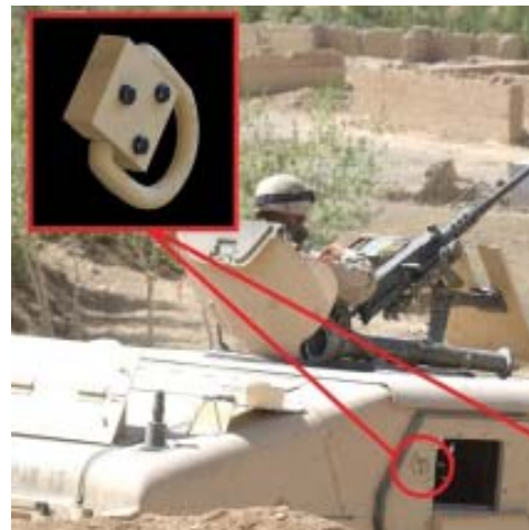
Aviation and Missile Research, Development and Engineering Center, Redstone Arsenal, Ala. The D-ring provides solid anchor points for the hooks of a tow strap, chain or cable to pull open damaged doors of an up-armored Humvee. U.S. Army photo
