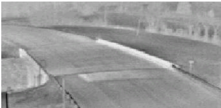
Fig. 7. Uneven heat distribution occurred with the original charge of HCFC-123 in all the heat pipes. Improvement was sought by replacing one evaporator section with HFC-134a and another with ethanol, with results shown here.
