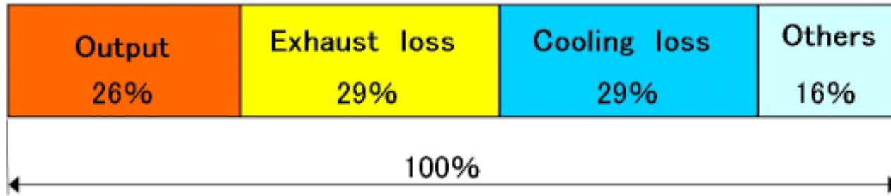
Fig. 2 Example of heat balance in a conventional engine
