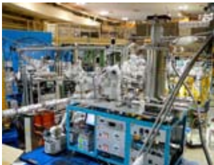
FIGURE 1. XAFS spectrometer equipped with a superconducting EDX detector system and energy resolution for the light elements at a KEK PF beam line.
