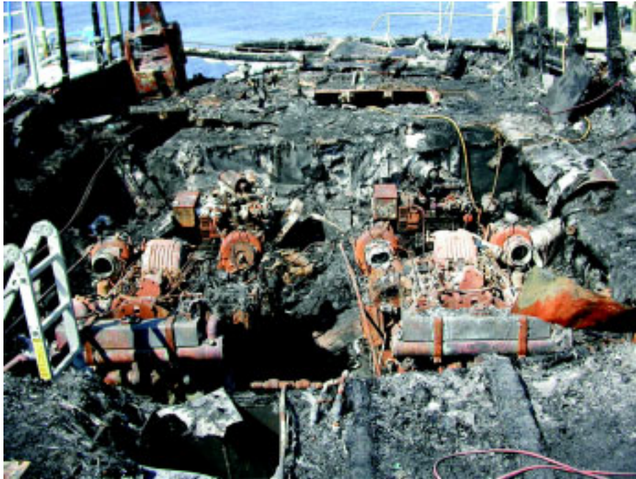
Figure 10. Looking aft toward the Express Shuttle II 's engine space after the fire. The starboard engine (left) was more severely damaged than the port engine (right).
