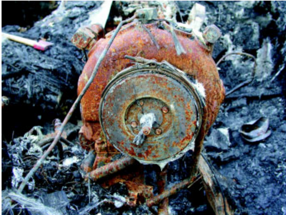
Figure 11. Photograph showing destruction on starboard engine's inboard turbocharger.
