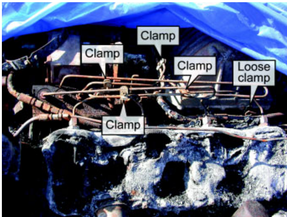
Figure 13. Photograph of fuel lines on the inboard side of the starboard engine block showing lines clamped together, and the loose clamp found between cylinders 5 and 7.
