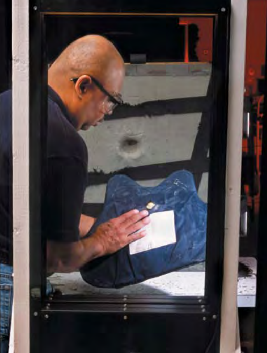
Nathaniel Waters, Office of Law Enforcement Standards (OLES), examines a bullet-resistant vest being tested. With funding from the National Institute of Justice (NIJ), OLES develops test methods and standards for the performance of equipment used by police, corrections officers and first responders. At the request of NIJ, NVLAP established a personal body armor testing laboratory accreditation program.
