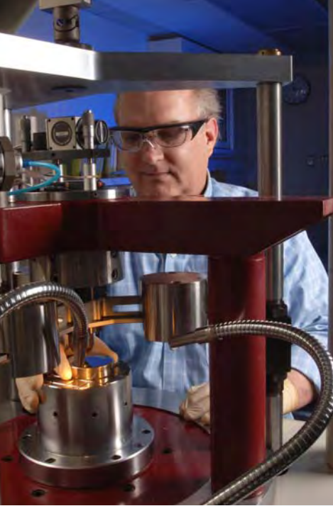
Sam Low, Metallurgy Division, in front of the primary Rockwell hardness reference machine for the United States. Sam Low is the Metallurgy Division's Quality Manager, and has provided continuing technical guidance in the area of hardness for both the NVLAP Calibration and the Fasteners and Metals Laboratory Accreditation Program.
