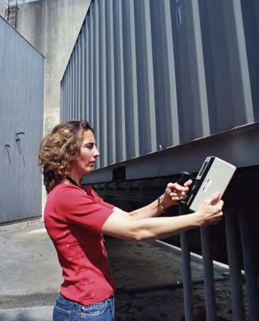
Leticia Pibida uses a hand-held radiation detection device to check the cargo of a truck trailer. She is coauthor of NVLAP's NIST Handbook 150-23 Homeland Security Applications: Radiation Detection Instruments.
