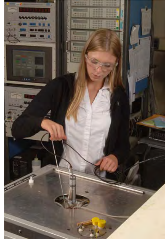
The Process Measurements Division at NIST Gaithersburg, MD, is in charge of realizing, maintaining, and disseminating the International Temperature Scale of 1990 (ITS-90). The Standard Platinum Resistance Thermometer (SPRT) Calibration Laboratory of the NIST Thermometry Group realizes the ITS-90 from the argon triple point (Ar TP, 189.3442 °C) to the silver freezing point (Ag FP, 961.78 °C) for the calibration of SPRTs. Michal Chojnacky, NIST physicist, is shown pulling the Tin Freezing Point cell out of its bath. Dean Ripple, Gregory Strouse, Karen Garrity and C. Dawn Cross from the division have all assisted NVLAP with calibration traceability, proficiency testing, calibration handbooks, and on-site technical assessment for those labs claiming the highest accuracies.
