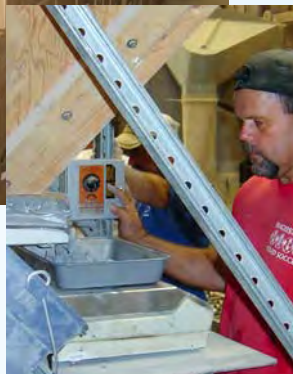
Shown in photo on the left are 3200 sample boxes of Coarse Aggregate to be shipped to participating laboratories as proficiency test samples. On the right, John Ardinger, AASHTO Materials Reference Laboratory (AMRL), is weighing out samples. More than 17,500 AMRL samples are sent out on an annual basis. About 1500 laboratories subscribe to the proficiency testing program of the Cement and Concrete Reference Laboratory (CCRL) and they ship about 7400 samples annually. The CCRL and the AMRL are Research Associate Programs located in the NIST Building and Fire Research Laboratory. CCRL is sponsored by ASTM and AMRL is sponsored by the American Association of State Highway and Transportation Officials (AASHTO). CCRL and AMRL operate proficiency sample programs that are required by NVLAP's Construction Materials Testing Laboratory Accreditation Program.
