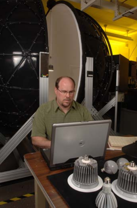
C. Cameron Miller, Optical Technology Division, in front of the NIST 2.5 m integrating sphere for LED measurements. Besides providing expertise and guidance on lighting proficiency testing, and selected on-site technical assessments, Dr. Miller is a technical expert assessor and coauthor of NVLAP's NIST Handbook 150-1 Energy Efficient Lighting Products.
