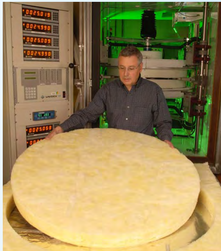
Robert Zarr, Building Environment Division, shown at the 1-meter guarded hot-plate apparatus that measures thermal conductivity of building insulation. This facility provides for absolute measurement of thermal resistance of thick and low-density test specimens used as transfer standards. These standards are used to calibrate heat-flow-meter apparatus (ASTM C 518) or verify guarded-hot-plate apparatus (ASTM C177). The division has provided technical support to NVLAP for the Thermal Insulation Materials Lab Accreditation Program.
