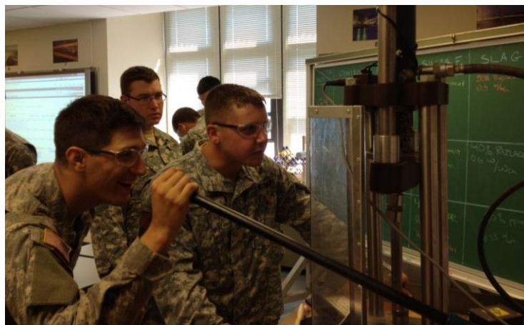
Pictured CE Firsties: CDT Seth Bell '13, CDT Gilbert Enzor '13 and CDT Peter Noto '13 conduct an axial compression test on their concrete cylinder at the start of Lesson 2 on 23 Aug 2012.
