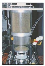
Millimeter-wave radiometer for measuring plasma electron temperature.
