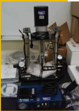
SprayWriter, for applying the repair material. © 2011 Florida State University. All rights reserved.
