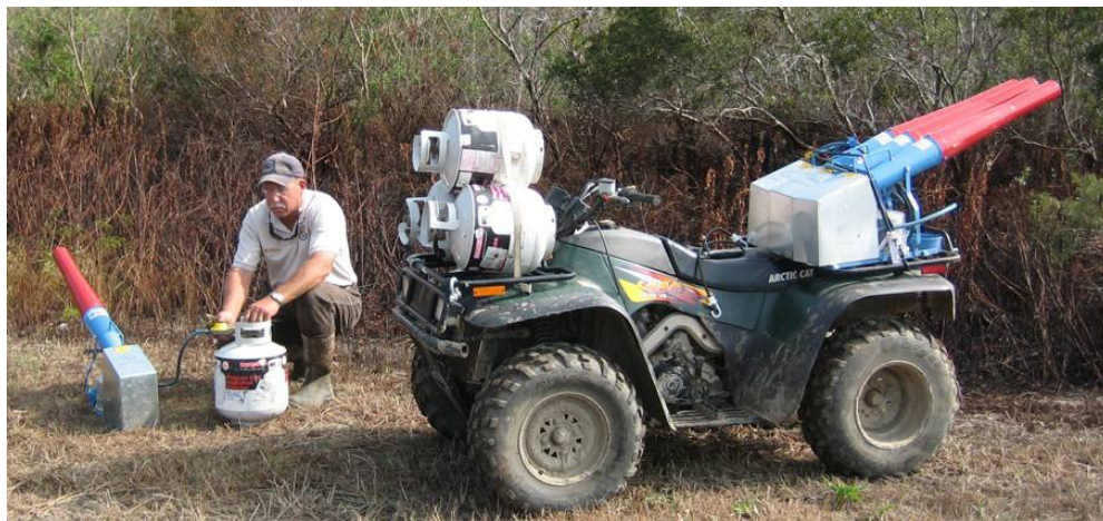
Environmental contaminants biologist deploys propane cannon to deter birds away from oil spill.
